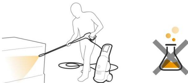
The container can be cleaned using a high-pressure hose. Only use soap and water, never chemical or abrasive products.
