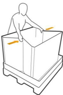
**1** With the lid off the container, push the sides of the container inwards at the crease in the centre of the walls, releasing the catches that lock it to the base.
