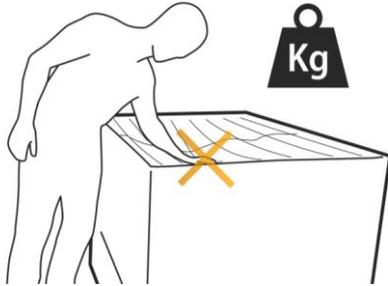
Never lean on or rest any load against the inside of the container. They are not designed for this and could break and/or become unusable.
