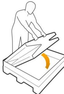
**2** Make sure that the folded walls are resting against one side of the base and lower them down gently, being careful not to knock the walls against the rim of the base. If the walls are suddenly dropped, the walls themselves or the rim of the base could be knocked and damaged.
