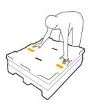
**1** Unlock the catches and remove the lid, lifting it by its handles. Leave the lid in a safe place, out of the way of vehicles or people.
