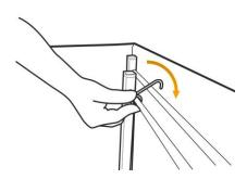
**4** Both frames must be fastened with the hook. Finish folding the container as described for the standard HybridBox.
