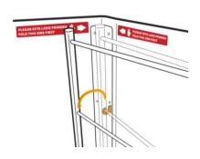
**1** To fold the container first unhook the frame from the side and fold it to the side stated on the label.
