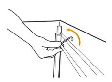
**1** First unfold the container as described above for the standard HybridBox. Once opened, release the hook the holds the frames together.
